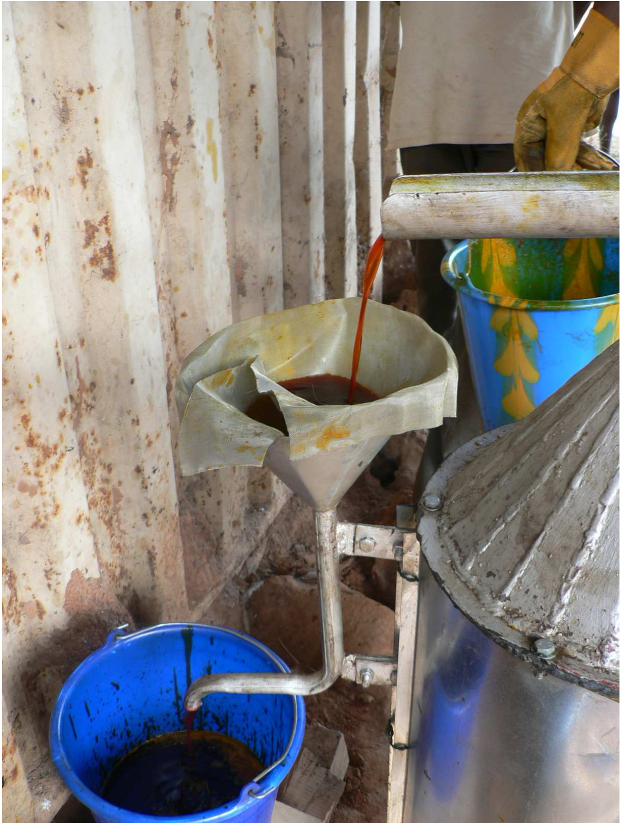
Palm oil at the exit of the Clarifier
